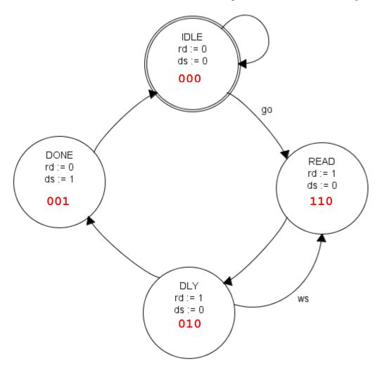
IDLE is 000, and READ is 110. Suppose we wanted the transition from IDLE to READ to be gray coded?
