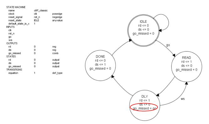
Notice the go\_missed output shows up on each state bubble with an "=" instead of a "<=", because it is of type "comb".
