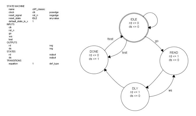
Since we expect test to be false during normal operation, we can just change the DONE->IDLE equation to "!test".
