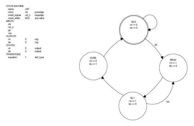
You might have noticed that I did not put an explicit "!go" on the IDLE loopback transition, nor an explicit "!ws" on the DLY to DONE transition. That is because fizzim understands that a transition with an equation of "1" is the default, lowest priority, transition. This will be explained in the section on transition priorities. You *can* add the explicit equations, but you don't have to.
